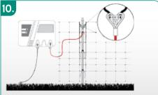
If possible, attach the fence connection cable to the metal clip. It can also be connected at any other point on the top strand.
